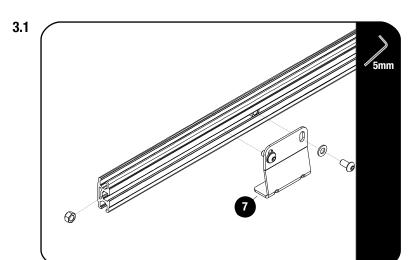
Loosely assemble the Mercedes Sprinter Feet (Item 7) using M8 x 16 Button Head Bolts, M8 Flat Washers and M8 Nyloc Nuts and slide them into the side profiles. They must still slide freely.
