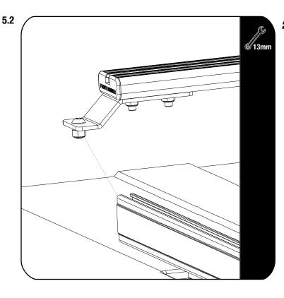
Slide pre-assembled Slats into the Side Profiles. Space the Slats at 404mm increments, or at your chosen spacing. These can be adjusted at any stage.
