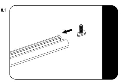
Slide four M8 x 20 T-Bolts (RRAC907) into the vehicles OEM tracks per side.
