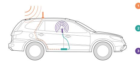
**Receives signal:** The powerful antenna reaches out to access voice and data signals, and deliver them to the booster.
