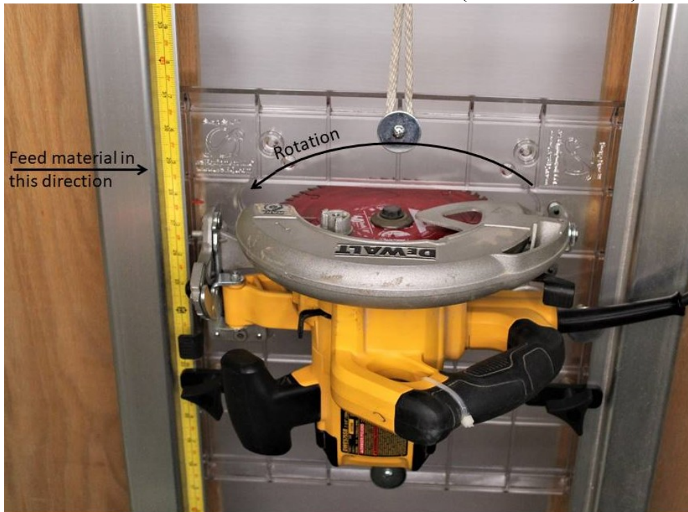
Adjust to the desired dimension and lock saw in place with both rail clamps. (Scale not included)
