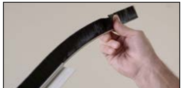
Capture brush into the aluminium carrier
