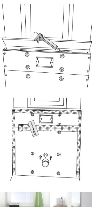
4) Cut out the cover and either bolt it into place or use PU assembly adhesive (e.g. JACKODUR<sup>®</sup> assembly adhesive) to glue it into place.
