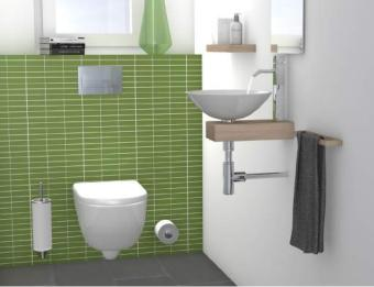
6) JACKOBOARD<sup>®</sup> Sabo must be covered with tiles to ensure the sufficiently even distribution of pressure when the WC is in use. The tiles can be laid directly on JACKO-BOARD<sup>®</sup> Sabo. All types and sizes of tiles can be used in principle. The tiles should, however, measure at least 100 x 100 mm, and be at least 7 mm thick. Once the tile adhesive has hardened, the WC can be mounted on the tile surface.
