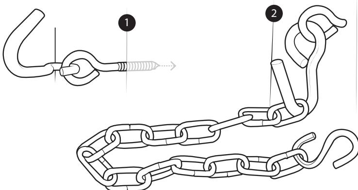
**EN** The best way to hang your hammock is with a Chain Kit. Screw the bolt hook into a solid upright beam. Two fixed points are necessary for hanging hammocks. The ideal position for these points: 3-4 m apart, 1.8 m high. Ensure a nice loose curve 30cm off the ground when sitting in the hammock.
