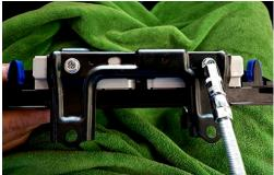
Insert the right side card of the armrest box, remove the original car bracket, and install it on the new screen assembly.
