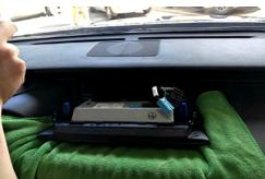
Remove the screen assembly and unplug the cable.
