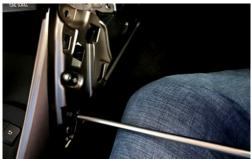
Remove the screws on both sides of the armrest.
