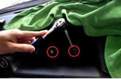
Use the warping plate to lift off the front baffle of the center control screen, and use the No. 10 sleeve to remove the two screws above.
