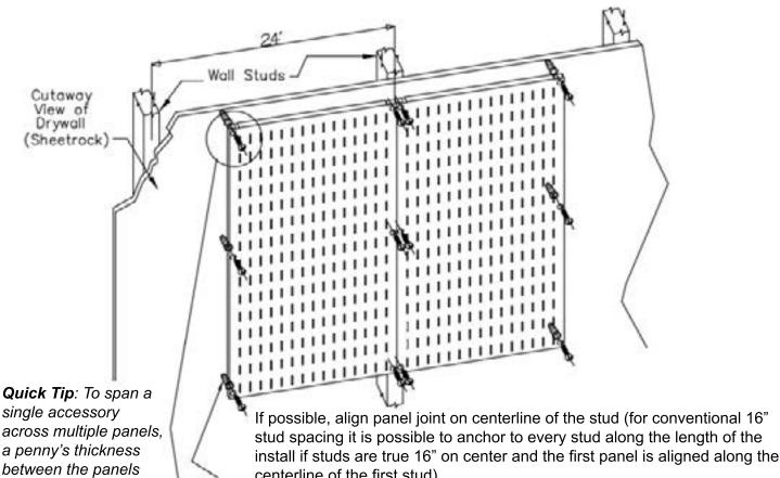
a penny's thickness between the panels creates the perfect spacing. Note, this is not required for any Wall Control accessory
