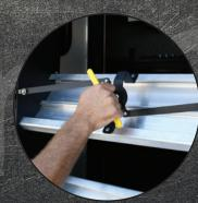
Easily turn the handle to release the steps, lower the lightweight steps to the ground, and enjoy solid entry to and exit from the RV.
