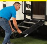
For uneven ground surfaces, remove pin on the extendible legs to adjust leg length.
