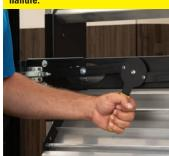
While holding the handle, release the SolidStep from the doorjamb. Slowly lower the step with both hands firmly supporting SolidStep.
