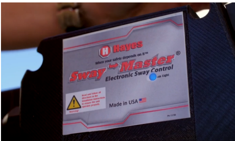
Fig. 8 – The status light will flash 3 times to indicate unit is activated.
