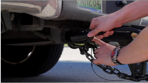
Fig. 7- Insert the Sway Master™ plug into the 7-way socket. Insert the trailer 7-way plug from the trailer into the Sway Master™ socket.
