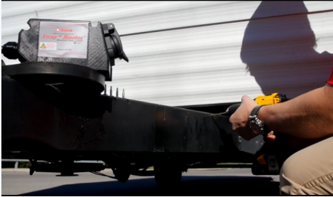
Fig. 3- Drill holes in trailer tongue
