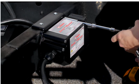
Fig. 5 – Using a 3/8" socket, attach Sway Master™ unit to the trailer with provided self-tapping screws.
