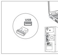
2. Take out the nano receiver from the color box and insert it into spare usb port of the computer
