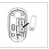
3.Put in AA battery and place it in correct direction (by following the sign of positive and negative indicated inside), and then turn on power on <on> poisition. Then close the battery cover.
