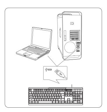
Insert USB plug of the keyboard into the USB port of your computer to work.
