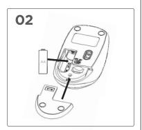
correct direction by following the sign of positive and negative indicated inside, and then slide power switch to position
