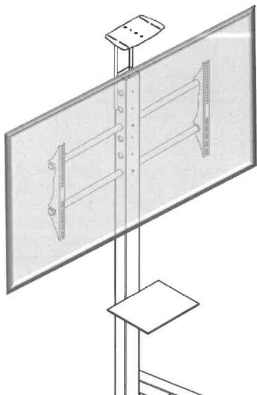
Install the screen on the FIX TROLLEY
