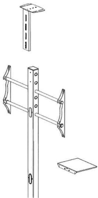
Insert the cables of your monitor inside the tube B through the oval holes and then cover the holes with the cap R
