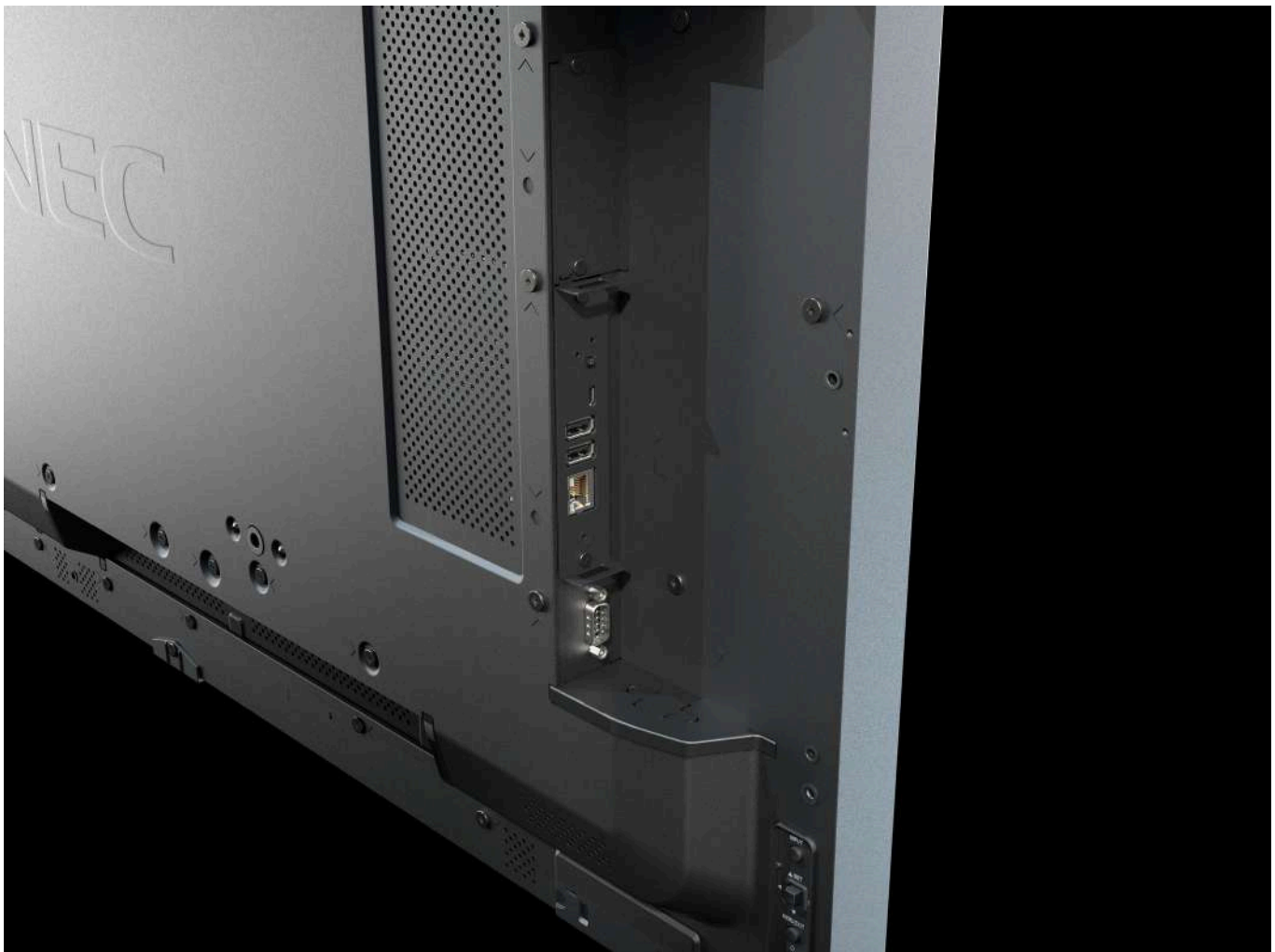
Final installed DS-IF20CE with RPI CM4 below
