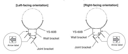
**Step 2.** Attach the joint bracket to the wall bracket using the supplied screws, adjust the horizontal speaker angle, then tighten the screws.
