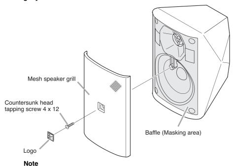
Because the logo is affixed using double-faced tape, peel it off carefully.
