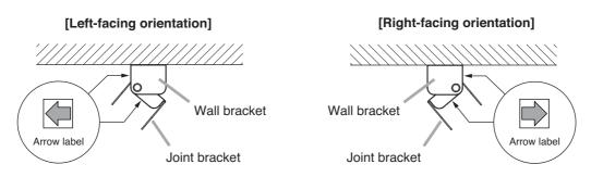
**Step 2.** Attach the joint bracket to the wall bracket using the supplied screws, adjust the horizontal speaker angle, then tighten the screws.
