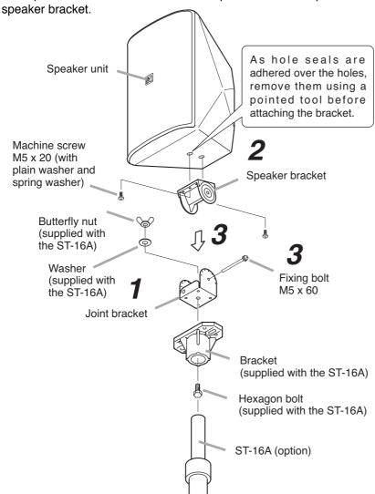
**Step 1.** Attach the joint bracket to the speaker stand bracket using the speaker stand's supplied bolt and nut.
