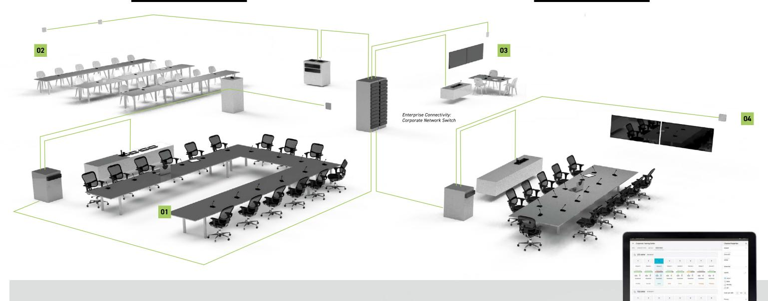
Microflex Wireless extends the Shure legacy of best-in-class audio to boardrooms, huddle rooms and meeting spaces, as well as education and training facilities of all sizes, delivering an enterprise-scale solution with confidence. All components in the Microflex Wireless system are connected and accessible over Ethernet networks. Any number of networked systems can be setup, managed, monitored and controlled on-site or remotely via web browser.
