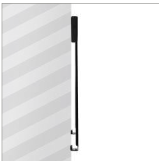
Low profile design mounts screen only 20mm from wall
