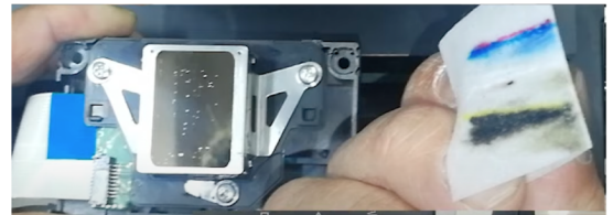
Use alcohol pads to clean printhead platen
