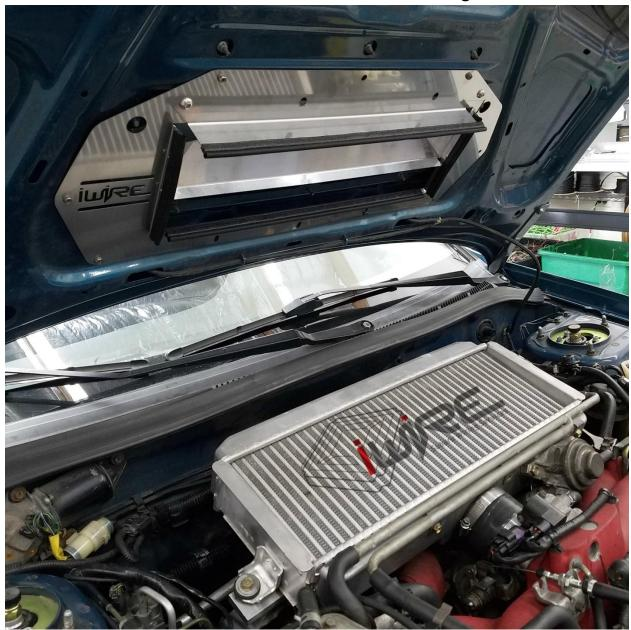
4. The gasket should not make contact with the intercooler itself but sit close to the fins (but not touching) and inside the outer housing.
