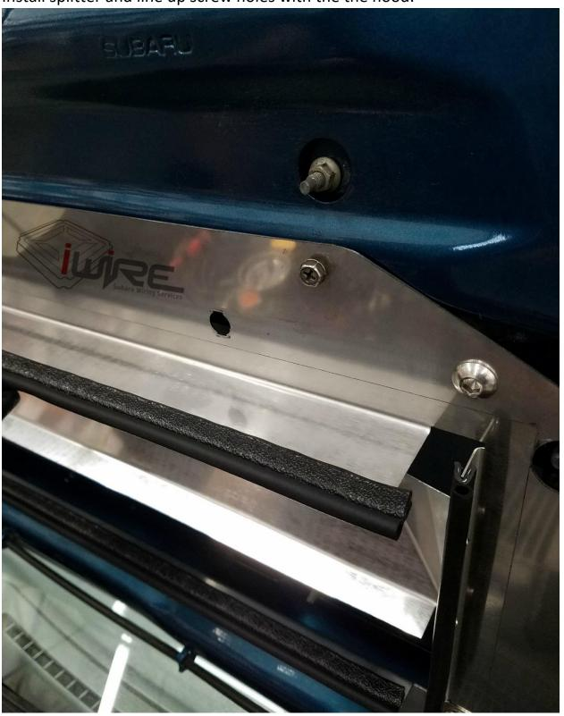
3. Tighten all screws down and attach clip. Lower hood slowly to verify proper fitment. The gasket should not make contact with the intercooler itself but sit close to the fins and inside the outer housing.
