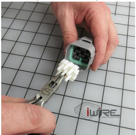
2. Insert the White, Brown, Yellow, and Orange in the order along the top row shown in the picture below. This will match the bulkhead side. Once completed pull gently on each wire to ensure they are seated then reinstall the lock.
