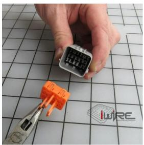
5. Insert the White, White Green, White Orange, and White Blue along the top row as shown in the image below. This will match the bulkhead side. Note this is the plug from the bottom side. Once completed pull gently on each wire to ensure they are seated then reinstall the lock.
