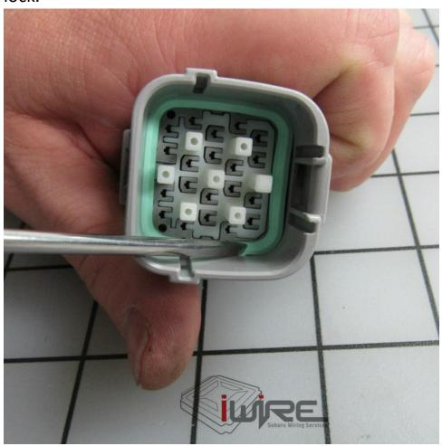
4. Remove lock of the Cam Crank Knock Receptacle. The lock will simply remove with a set of pliers. Pull on one of the protruding pieces of the lock with a set of pliers. The lock should pull out with a firm tug.
