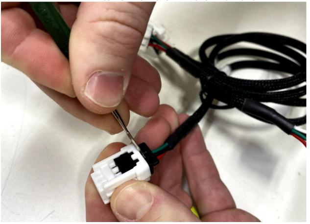
Slide the pick in to lift up the tab. A video about depinning techniques can be found here
