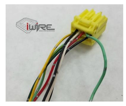
**For V5 to V6 RHD** – Tap into the Light Green wire on pin 20 in the Blue plug for throttle position at the engine computer.
