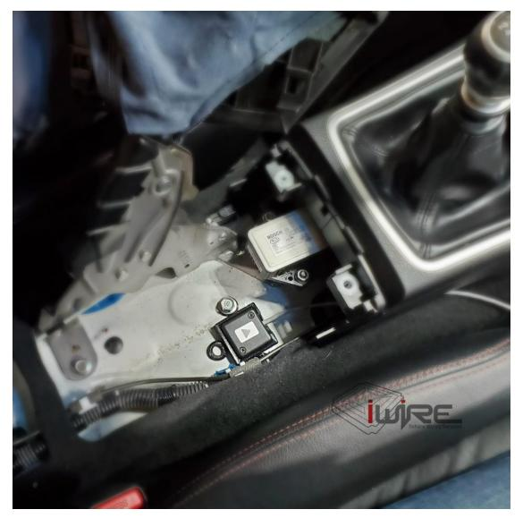
6. **Ground the ring terminal** from the Green wire (item 5 in kit). This ground ring terminal can go to any bolt in the car. We suggest routing it to either the bolt that holds the G Sensor below the Ebrake or a bolt on the dash bar. Please note – if there is paint on this bolt you're using for your ground you will need to sand it for better contact. You want metal to metal contact here for the best ground possible.
