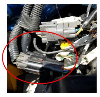
Another view of the connector from the transmission adapter to the original transmission harness in the car.
