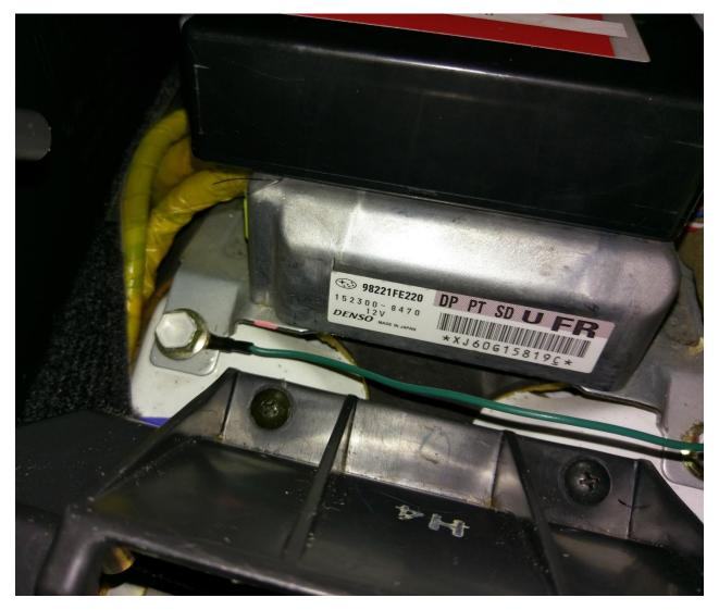
6. **Tap the Throttle Position Sensor Wire** (Blue wire – item 4 in kit). This step is for DCCDPro Spiider controllers only. If you have a Manual controller you will not complete this step.
