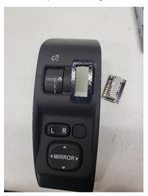
Then slot in the LED into the back. You can use a dab of glue to secure it to the mount.
