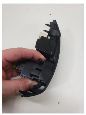
The next step is to mark where the opening will be slightly enlarged to fit the LED. Place the holder in the opening and the then mark the spot where you the trim panel is still seen.
