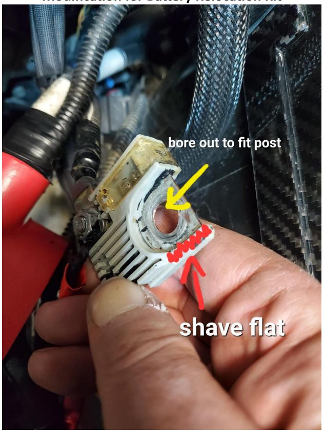
2015+ WRX Electronic Power Steering Fuse Modification for Battery Relocation Kit
