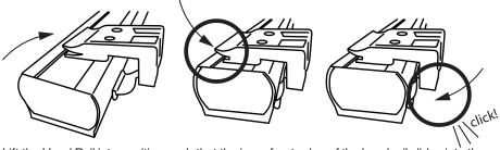
Lift the Head Rail into position such that the inner front edge of the head rail slides into the slot at the front of each bracket (see illustration), and then push the head rail upward until the flexible tab at the bottom of each bracket snaps onto the back of the head rail. Check carefully to assure that each bracket is properly secured.
