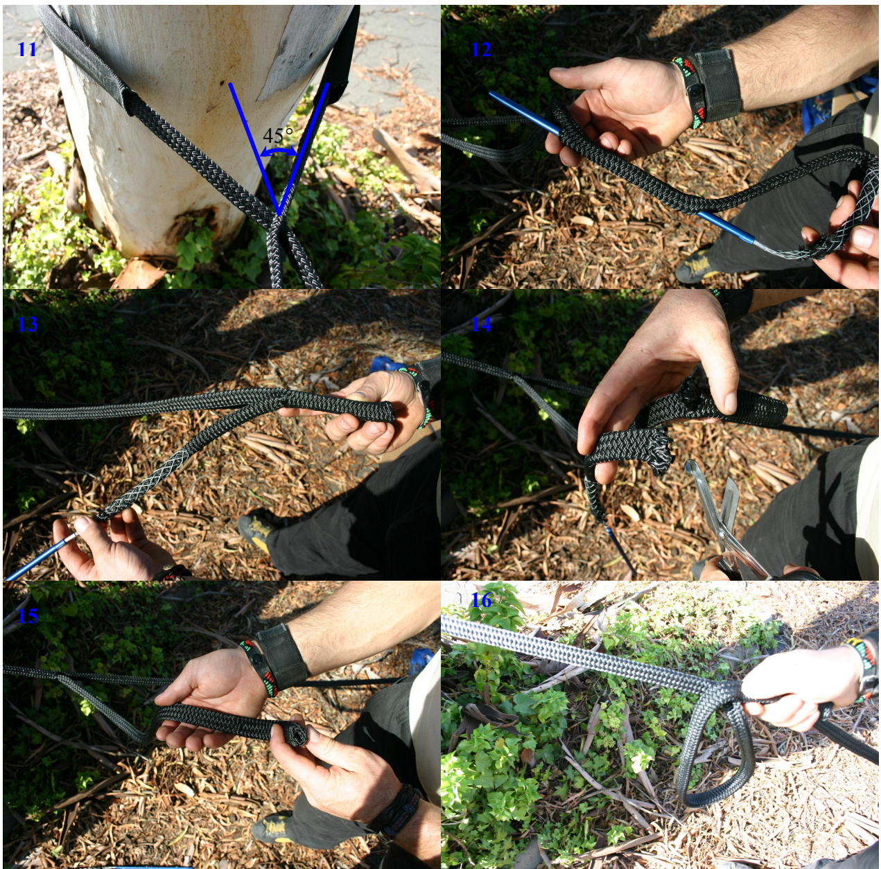
Figures 11 - 16: Finishing Off Splice
