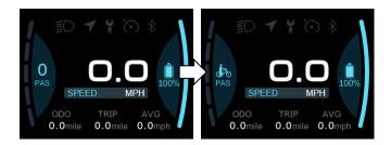
In the push mode, the boost logo is dynamically displayed, the vehicle speed is less than 6km/h, the push state is stopped, the screen boost logo disappears and the static boost logo state is restored. Under static boost, no button press within 5s is automatically adjusted to 0 gear.
