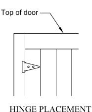
19. The hinge pin should sit right over top of the seam between the door and the door trim. Using the 1/8" drill bit pre-drill holes before mounting the hinge screws. First mount hinges to the then use the door spacer shim supplied, to raise the door above the front floor trim to the proper clearance height then mark the screw locations on the door trim. Pre-drill with 1/8" drill bit then mount door to the front.
