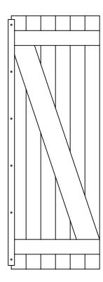
20. Using the 1/8" drill bit, pre-drill the holes on the door stop before mounting on the door. Use about 6 - 1 1/8" nails to affix the door stop to the door.
