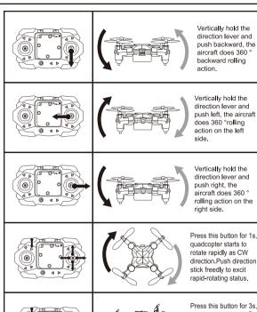
Press this button for 3s, quadcopter starts to fly as a CW circle.Push-direction stick freedly to excit circle-flying status.
