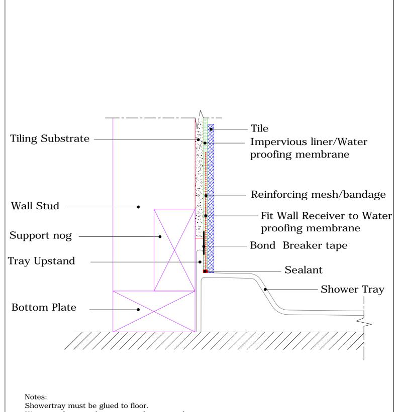
Waterproofing membrane to overlap upstand.
