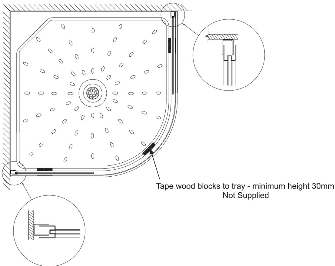
Lift Door Frame assembly onto the wood blocks and place into Wall Receivers as shown
