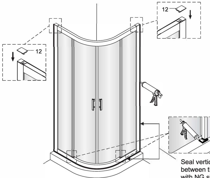
Seal vertically up each Wall Receiver and between the Sill and Upstand of the tray with NG silicone sealant
