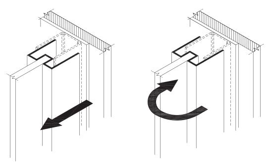
While still resting on the wood blocks "Spring" the Door Frame assembly so it sits over the legs of the Wall Receiver. Repeat for other side.
