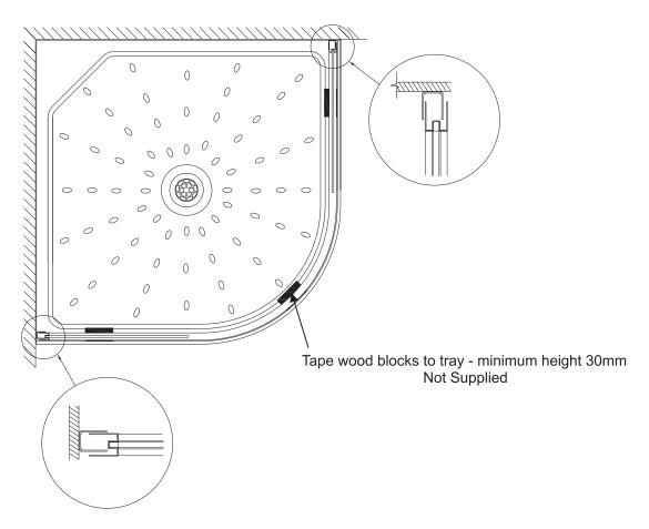
Lift Door Frame assembly onto the wood blocks and place into Wall Receivers as shown When lifting the Door Frame assembly, hold it by the vertical edges of the glass or door frame. Under no circumstance lift by the Head and Sill as this may cause the glass to fall out of the glazing gaskets
