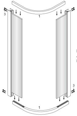
Make sure to tighten the screw. Any gap or clearance will result in leaking issue.
