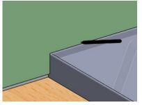
7. Remove the tray and cut out the rebate in the Plasterboard
