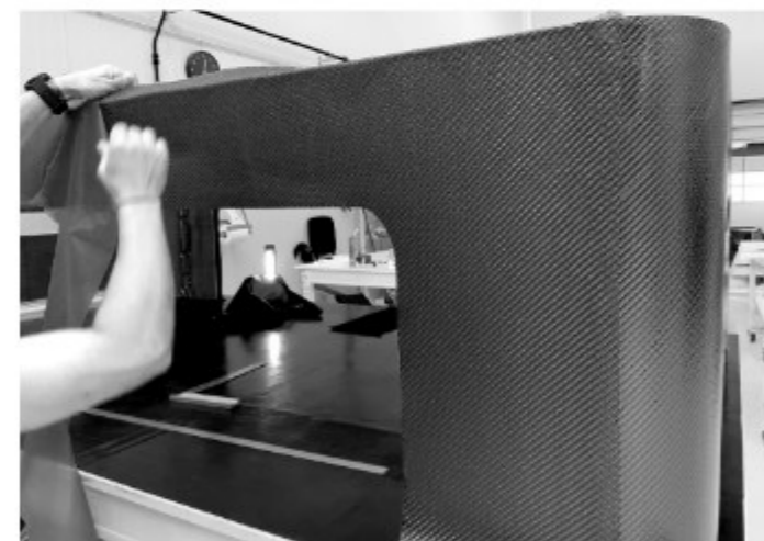
Outside skin manufactured 100% in carbon fiber prepreg, aeronautical grade, with pvc core
