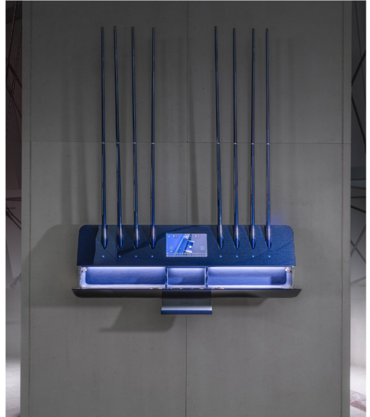
Siemens Simatic HMI Touch high resolution 13" control panel, located in the wall cue support.
