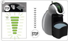
The bar display and power button are blinking green at the end of the descaling cycle.
