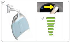
Check if there is water in the water tank: if not, refill and press hot/cold button again to continue preparation; if the water tank is full proceed as follows:
