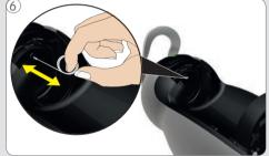
Unblock the injector with the cleaning needle.
