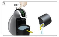
Wait until machine switches back to normal operation. Then switch off machine. Remove and empty capsule bin.
