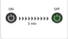
After 5 minutes of non-usage the machine automatically shuts down (Economy Mode). To restart, press power button.
