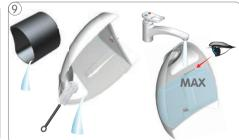
Empty capsule bin. Rinse and clean water tank thoroughly. Fill water tank with fresh, drinking water up to max. level.
