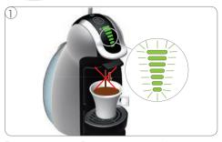
Error symptoms: Beverage preparation stops part way during delivery or does not start at all. Bar display flashes and power button blinks red and green rapidly.
