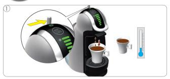
If the beverage only comes out in droplets or if the beverage is cooler than usual, the machine has to be descaled.
