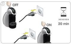
(see page 12). Unplug power plug and wait 20 minutes. Afterwards plug power plug into mains power socket and switch machine on.
