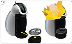
Place drip grid on drip tray. Then insert drip tray at desired position of machine. Clean machine with a soft damp cloth. Dry it afterwards with a soft dry cloth.
