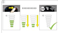
Move the lever to the right for hot beverages and to the left for cold beverages. Beverage preparation starts. Bar display lights vanish progressively. Machine stops preparation automatically. Extraction can be stopped manually by moving the lever back to the middle position.
