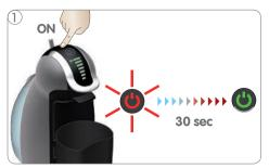
Switch machine on. While machine is heating up, power button starts blinking red. After approx. 30 seconds, power button lights steady green and machine is ready.
