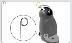
Remove the water tank and take out the cleaning needle. Close the locking handle.
