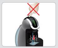
Do not push power button during descaling cycle.
