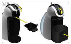
Open locking handle and insert empty capsule holder. Close locking handle and place capsule bin under the delivery outlet.
