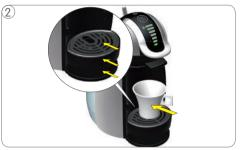
Adjust drip tray position according to the chosen beverage (see page 6-7). Place cup on drip tray.
