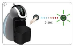
Press and hold power button for at least 5 seconds. Power button starts blinking green and machine enters the descaling mode.
