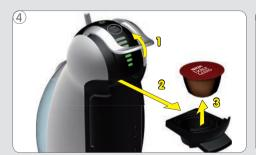
Then lift the locking handle and remove the capsule holder.
