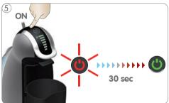
Switch machine on. While machine is heating up, power button starts blinking red. After approx. 30 seconds, power button light turns green and machine is ready to use.
