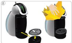
Place drip grid on drip tray. Then attach drip tray at desired position on machine. Clean machine with a soft damp cloth. Dry it afterwards with a soft dry cloth.
