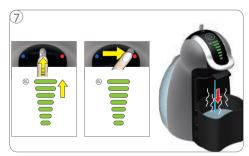
Push the lever up to set the bar display to maximum level. Move lever to the right for hot extraction. Bar display begins to count down. Machine descales in start-stop operation for approx. 2 min.
