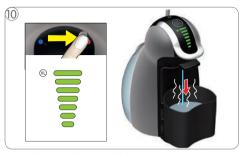
Move lever to the right for hot extraction. Bar display begins to count down. Wait until machine stop, bar display and power button start blinking green.
