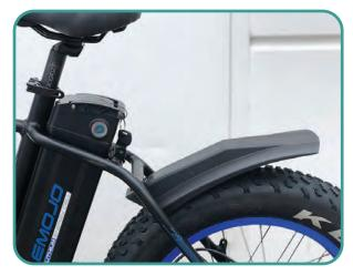
2-Mounded on the frame. Fix the fender to the frame rear end crossbar.
