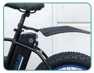
1-Mounted on the seat pole. Attach the round clamp end to the sea pole and the other end to the fender using the provided screws.
