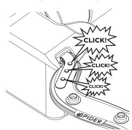
For camera utilizing an eyelet connection, install one of our provided adapters.
