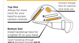
1. Insert the hand strap through the adapter slot and fold.
