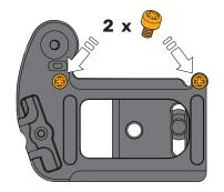
For small bodied **DSLR CAMERAS** and **MIRRORLESS CAMERAS WITH BATTERY GRIPS**, remove the two screws as shown.
