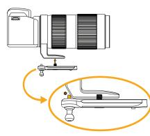
\*Lens Plate RAISED FEATURE must be in contact with the back of the lens collar.
