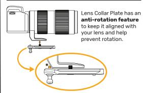
Lens Collar Plate's RAISED FEATURE must be in contact with the back of the lens collar.
