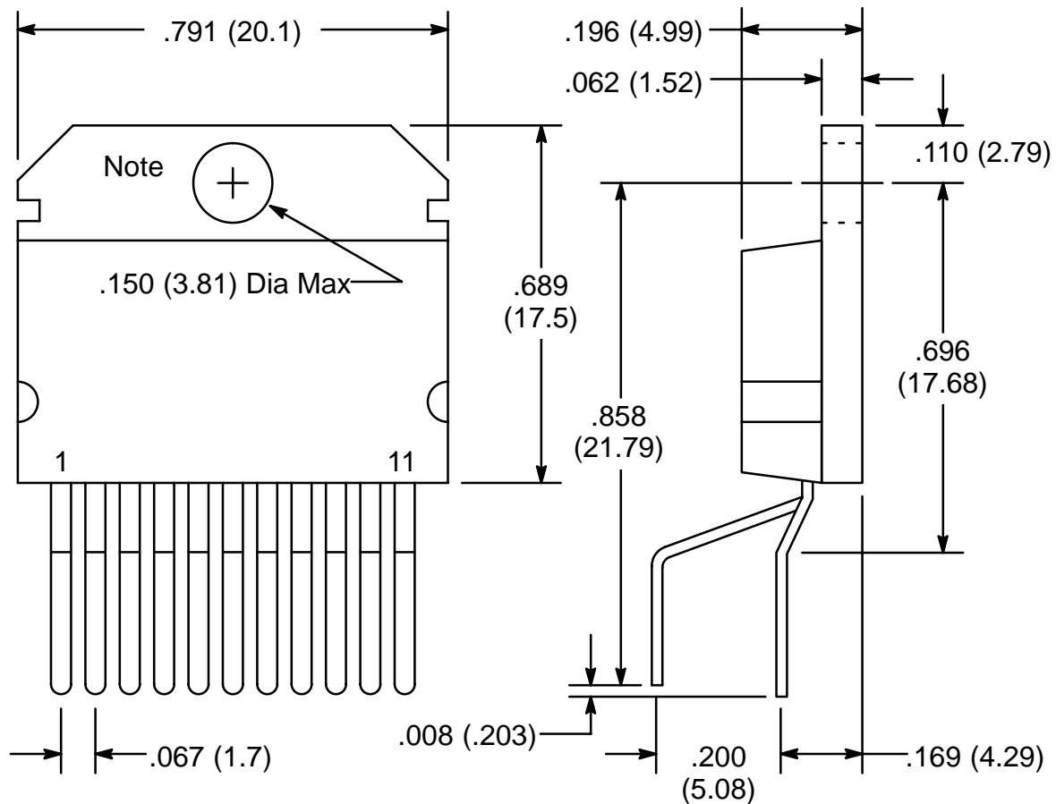
**NOTE:** Tab connected to Pin6
