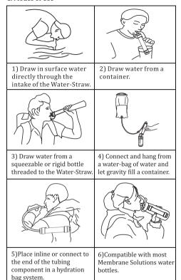
(Note: if the ultrafilter fibers are wet, then it's important to make sure there is no air gap between the fibers and water. The ultrafilter module must be flooded in order to allow drawn or pressurized flow through the filter.)
