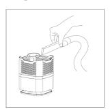
Clean out any accumulated dust, lint, or hair inside the air purifier using a vacuum hose of dry cloth.
