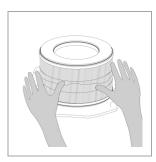
Remove any packing material from the new filter element.
