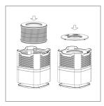
Slot the new filter into the base of the purifier. Replace the filter cover and twist in the closed direction to lock it in place. Turn the purifier upright. Plug in the air purifier and follow the Filter reset instructions (See Page 10).
