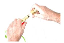
NOTE: To remove the hose from the "Y" connector first press in the blue locking collar before pulling the hose.
