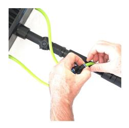
To extend the pole, first un-clamp the green pole clamp (closest to the bottom of the pole) and extend. Then lock the clamp and the extend the other sections one by one.
