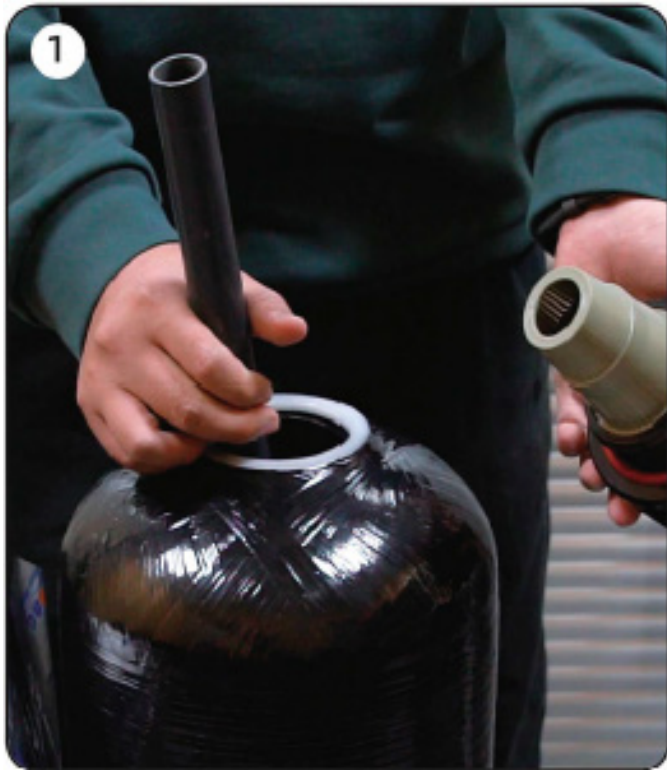
Pull out the riser tube
