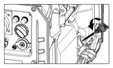
4. Tilt the generator on its side and allow the oil to drain completely.
