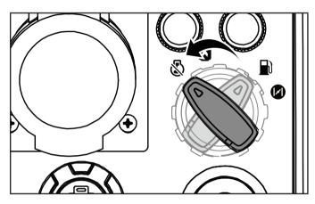
**Important:** Always ensure that the dial and fuel vent on the fuel cap are in the "OFF" position when the generator is not in use.
