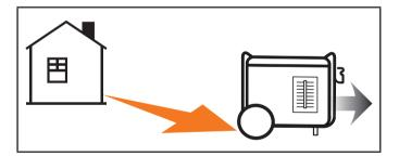
If misused and operated in an unapproved and unsafe location that results in the accumulation of poisonous CO gas inside an enclosed or partially enclosed space, for example a house, garage or a garage with the door partially open, CO Shield<sup>®</sup> will automatically shut off the generator and then will illuminate a blinking red LED light. **Read the action label for next steps.**
