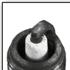
Spark plug has dry deposits
