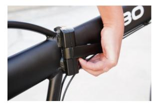
Step 2: Push the button on the headtube latch to release it and unlock the folding mechanism.
